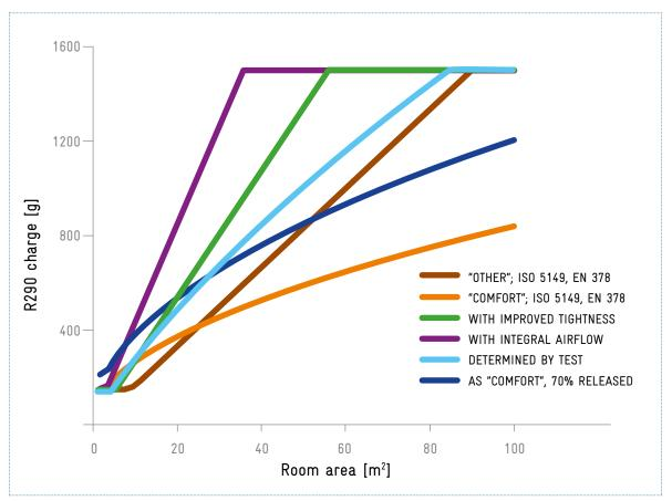
(Note the "installation height" for air conditioner and improved tightness is 2 m and the curve for "determined by test" is approximated based on tests with an air conditioner indoor unit at 2 m.)
