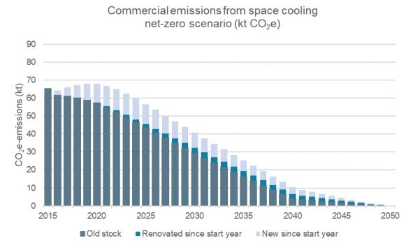
Figure 28.  $CO_2$  emissions (direct and indirect) from space cooling of the commercial sector in the netzero by 2050 scenario.
