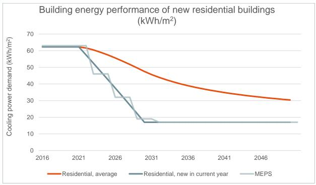
Figure 7. Energy performance per square meter for new residential buildings in the Enhanced ambition scenario.
